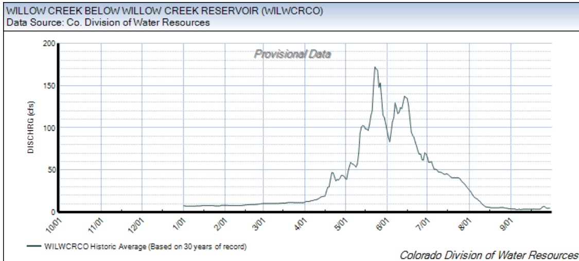
Figure A.5 – Average annual hydrograph for Willow Creek below Willow Creek Reservoir based on 30 years of record.
